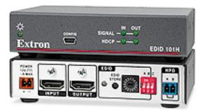
It communicates pre-stored EDID to the source according to user-selected resolution and refresh rate, and also captures and stores EDID information when connected to a display.
