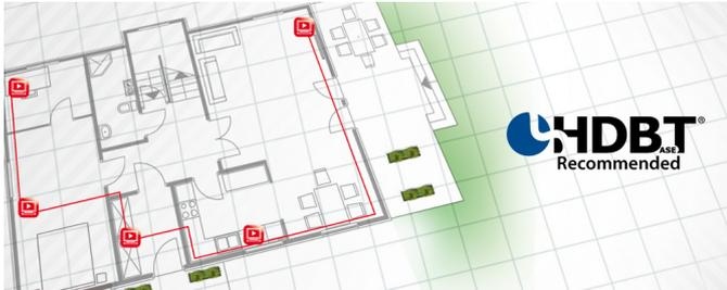
Tested and certified by the HDBaseT Alliance, the cables are ideal for high speed data networks across homes or buildings. As one knows, the HDBaseT standard allows HD video, audio, ethernet, power and control signal distribution over a single cable for up to 100m.
