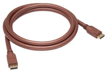
Copper cables carrying high resolution DisplayPort cables over long distances must overcome several challenges, such as insertion loss, differential skew and jitter. Insertion loss is caused by cable capacitance acting as a low-pass filter, blocking higher frequency signal components. Skew occurs when differential DisplayPort signals get delayed and become out of phase when passing over a lang cable.
