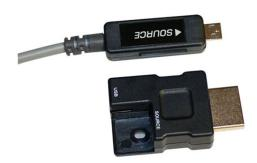
The P-HDFH-DC2 Active Optical cable is a plenum-rated, flexible cable with a 5mm bend radius. It is constructed using fibre optics, and as such can be offered in much longer lengths than standard copper HDMI cables. It also has detachable connectors, allowing installers to easily pull in the cable in tight spaces or through conduits.
