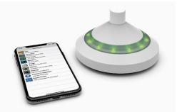
The dBPod features coloured LED lights providing a clear visual status in real-time, together with a companion app for more in depth data. To do so it uses a MEMS wideband omnidirectional microphone coupled with an audio interface, a microprocessor, flash memory, a lithium ion battery and an audio jack to create a powerful measurement tool.
