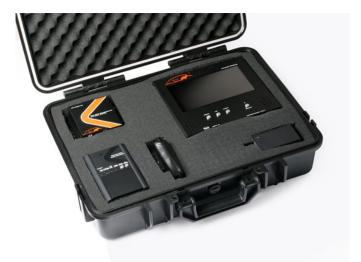
The company says the kit diagnoses 99% of all A/V digital connectivity issues (saving installers time and overhead) through its combination of portable HDMI signal generator, 7" HDMI monitor, EDID emulator and 5-hour monitor battery inside a high-quality Pelican case.
